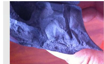
Inside section of blades white parts is carton fiber material
